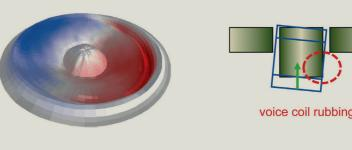
Rocking mode is usually the first circumferential mode which may cause voice coil rubbing. Check that AAL of the quadrature or circumferential component is at least 10 dB below the total AAL!
